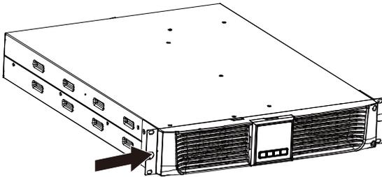
2. Assemble the rack rails with the rack-mounting.
