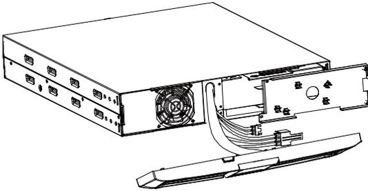
5. Pull the battery pack out onto a flat surface.
