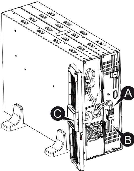
● **Connecting the EBM in a rack form**
