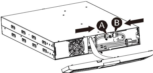
8. Re-install the front panel on the UPS.
