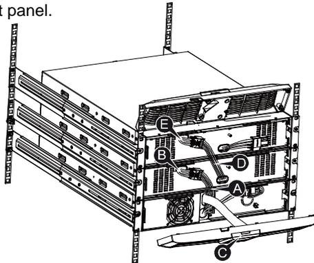
**Note:** Three or more EBMs can be connected to the UPS in the same way as shown above.
