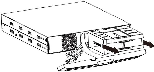
6. Install the new battery pack into the UPS.
