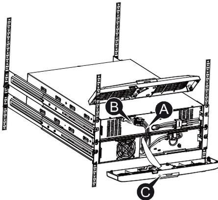
5. After installing the UPS into the rack, the load can then be connected to the UPS. Please make sure the load equipment is turned off before connecting all loads into the output C13 ports.
